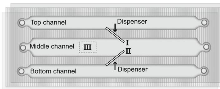
**Fig. 2** Microfluidic chamber design. The solutions flow from *left to right*
